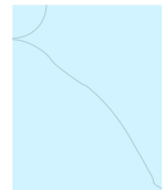
Bending Break Pattern: This type of pattern is seen when someone tries to open a locked window. It comes from racking of the sash when this action occurs it can cause a break.
