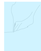
Thermal Stress Break Pattern: This occurs when the center of the glass becomes warmer than the peripheral. When this difference exceeds the tensile strength of the glass it will break. It is easy to identify this pattern since the glass will break straight out for an inch or so then have a normal break pattern.
